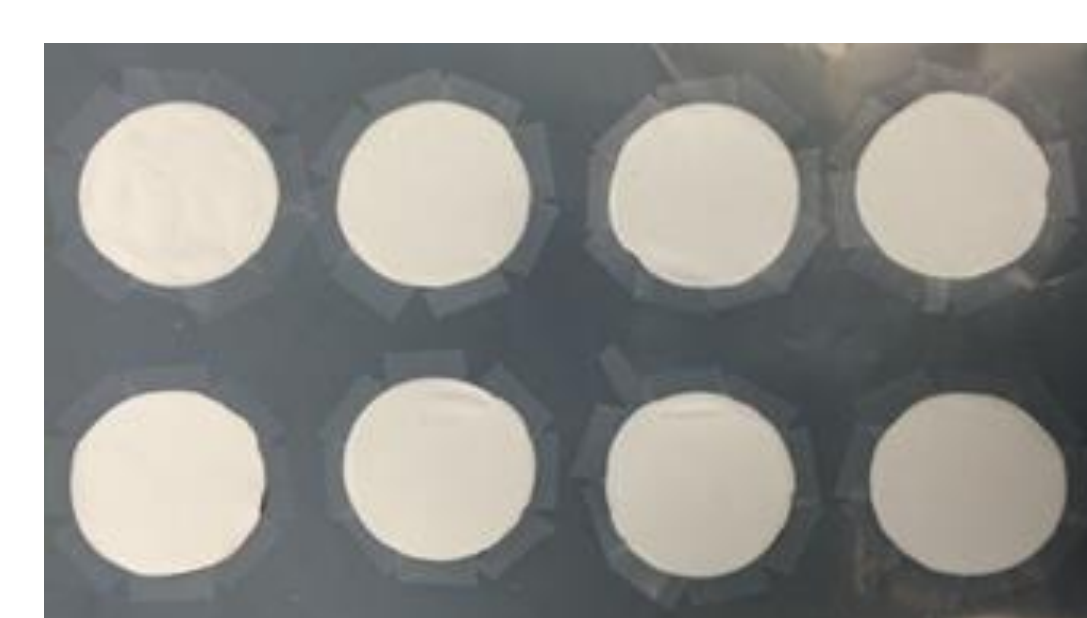
Template support for the filter disk substrates to be CL coated by Mayer bar
